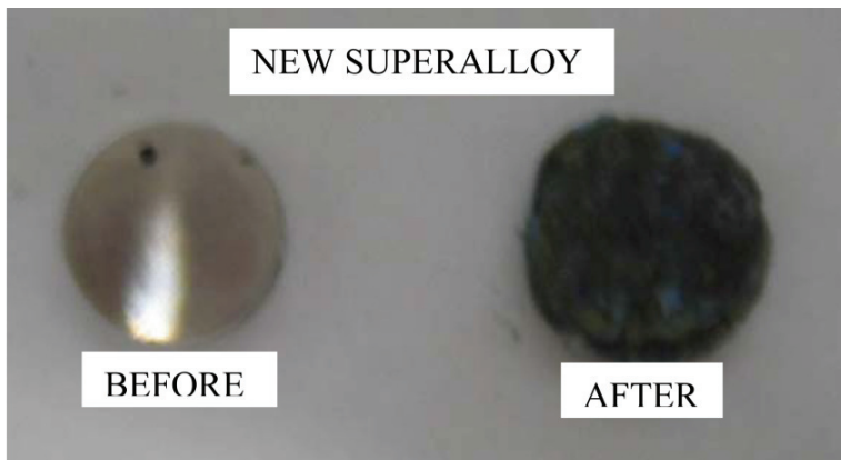
Fig. 8. Before and after hot corrosion in marine environment under type I conditions
